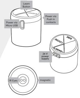
Be aware of the correct positioning of the connectors on the power meter.
